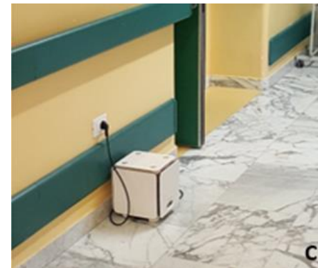
Three JONIX cube devices with NTP technology placed in hospital wards in Lombardia where the test was carried out.
